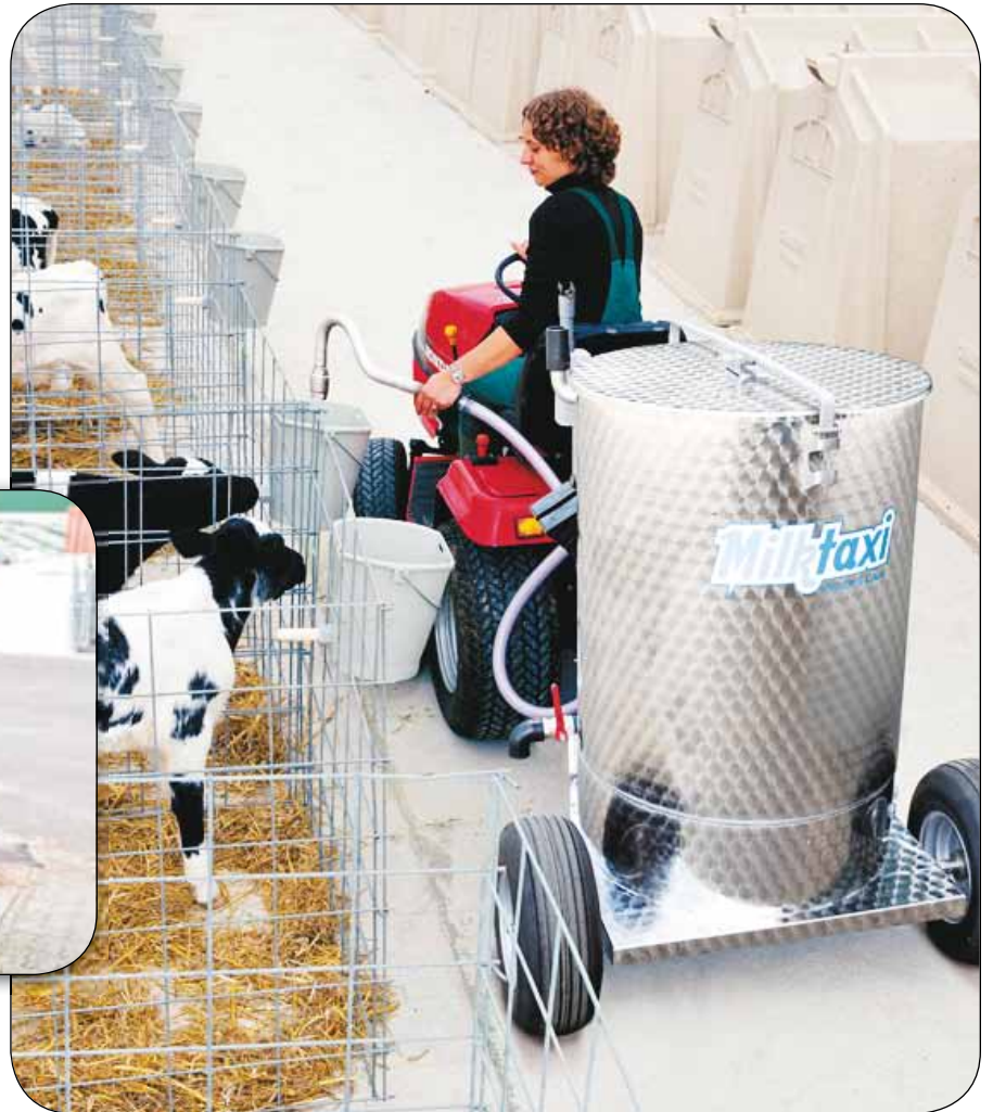
A metered dosing pump lets calf feeders walk or drive by calf pens and deposit the right amount of milk every time. The Milk Taxi is shown here. Photos courtesy of Calf-Star.
